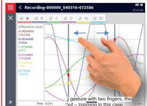
Figure: Using the magnifying gesture with two fingers, the operation is carried out – zooming in this case
