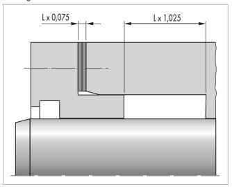
Adjustable housings have the advantage of an optimal adjustment option for the sealing effect with minimal idling friction.
