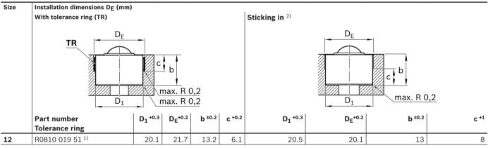
1) Made from corrosion-resistant steel 1.4310
