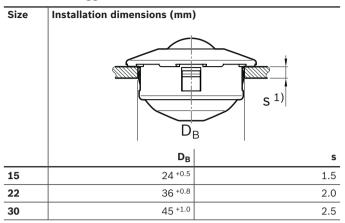
1) Minimum thickness of the mounting plate
