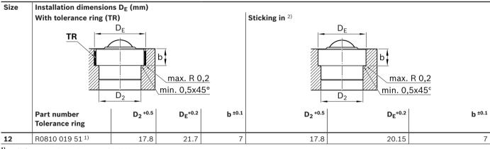
1) made from corrosion-resistant steel 1.4310
